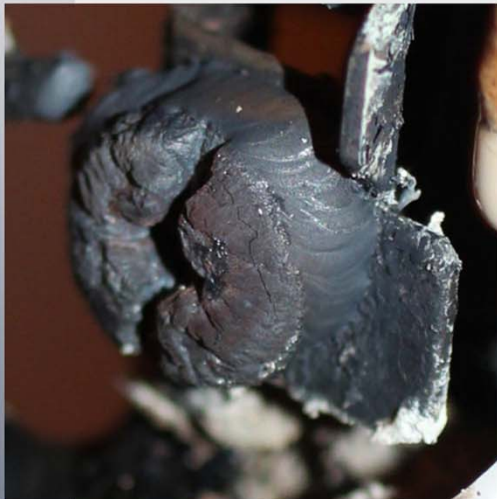
Welded Conductor w/Curved Striations
